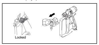
2. Close the paint valve (D or E) for the gun to be flushed. Fig. 1.
